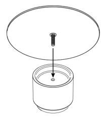
Guide the threaded insert into the hole on the tingle base and turn clockwise to fasten
